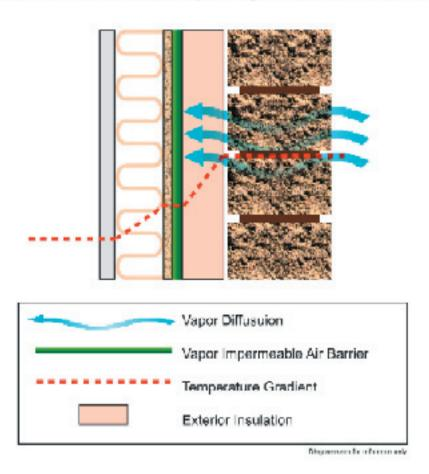
Moving north to, say, Boston, things get more complex due to the seasonal variations in both temperature and relative humidity. However, the most dramatic temperature gradients are generated in the cold months, when the air is warmer inside the building structure and colder outside, creating vapor drive inside to outside.
