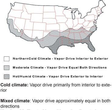
Hot, humid climate: Vapor drive primarily exterior to interior
